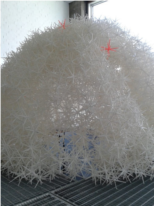
Figure 1: Aggregate Structure – Cantilever dome of granulates
