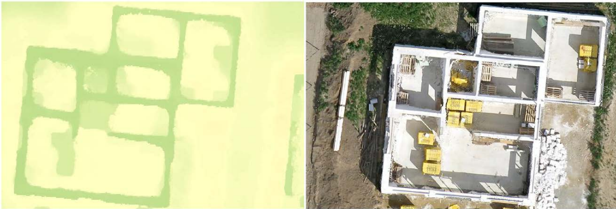
Figure 2: Detail of the difference of DEMs between two epochs and a corresponding orthoimage
