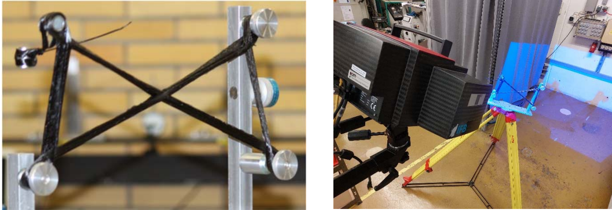
Figure 3: Measurement Set-up for TLS measurements without scanning spray (left). Measurement set-up with ATOS System (right).
