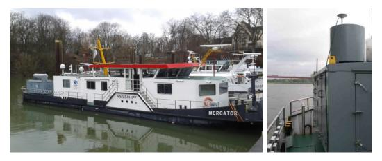
Figure 4: "Mercator" observation vessel for the measurement data (left figure); GPS antenna over the vessel (right figure)
