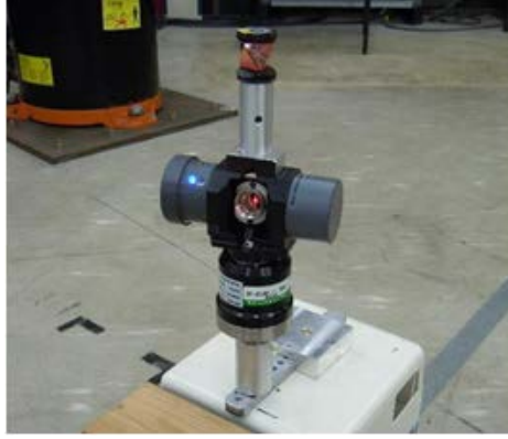
Figure 5: Target Device Combination: Active Target and 360° Prism GRZ101
