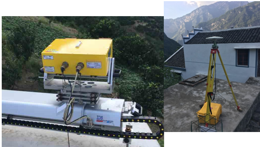
Figure1: Ground-based SAR and GNSS measurement at Three Gorges Dam
