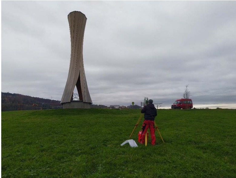
Figure 5: Network measurement when measuring the fixed point network
