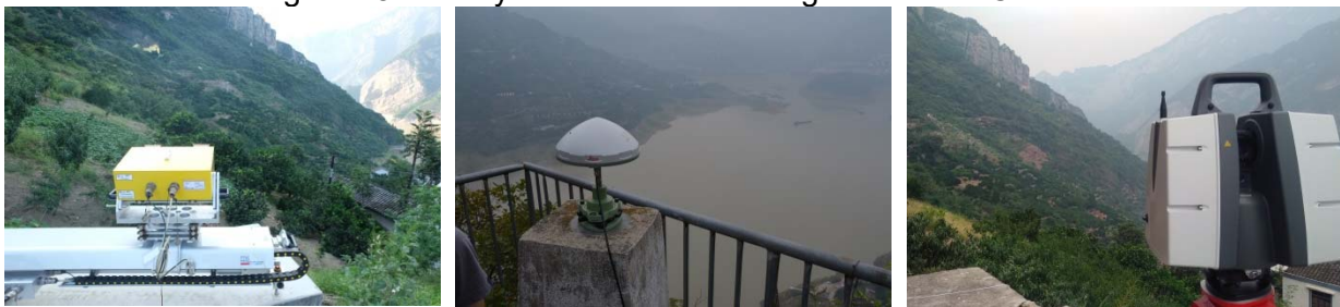
Figure 19: Instruments used for the deformation measurements. From left to right: GB-SAR, GNSS-receiver and TLS
