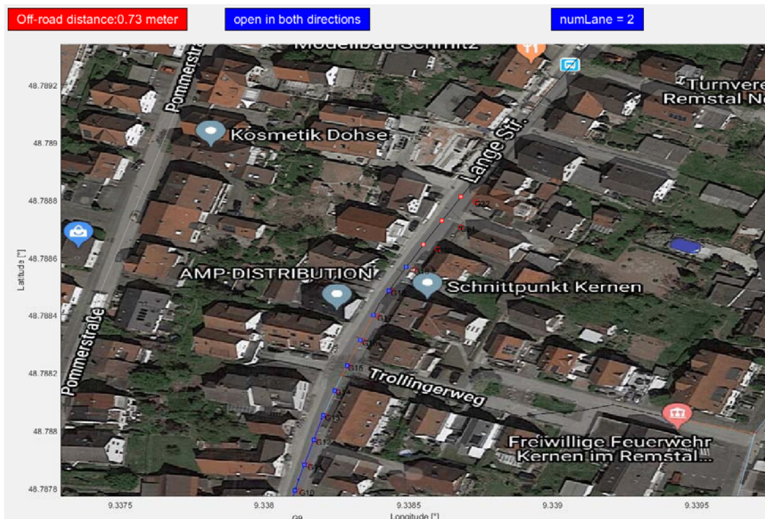
Figure 15: An example of map-aiding result with off-road estimation
