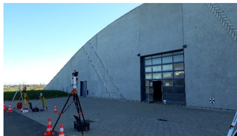
Figure 6: Measurement setup at Bonn reference wall.
