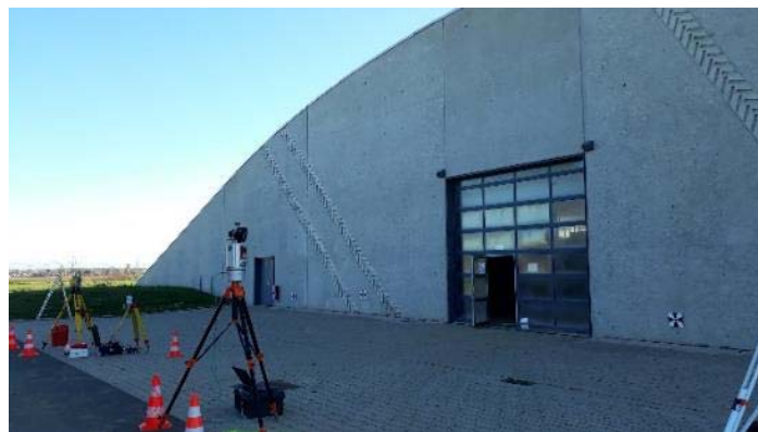
Figure 4: Measurement set-up at Bonn reference wall
