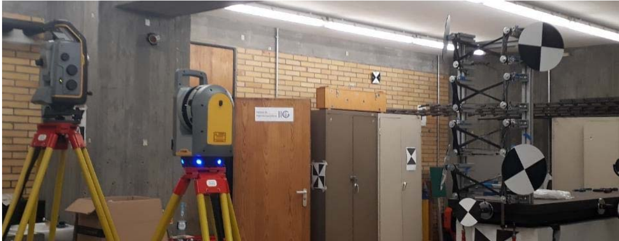
Figure 2: Measuring set-up for the geometric quality control after the production.
