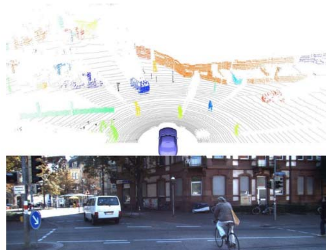
Figure 10: Segmentation of lidar scan into point cloud segments using a geometric approach
