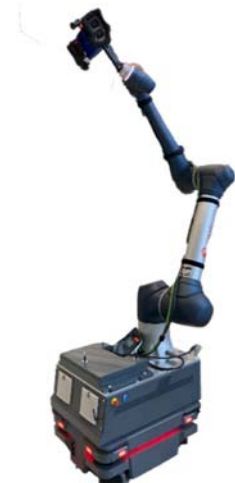
Figure 11: SME-SL for automated gap- and flush measurement
