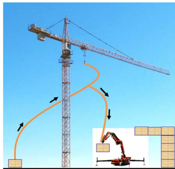
Figure 2: Example of the cooperation between two cranes for the automated/partly automated construction
